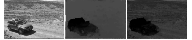
Fig. 5. The left image is one frame from the "jeep" sequence. The middle image is the optical flow intensity map as the reference frame. The right image is the destination image.
